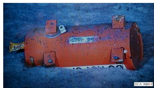
Protected part of the FDR without its ULB beacon
