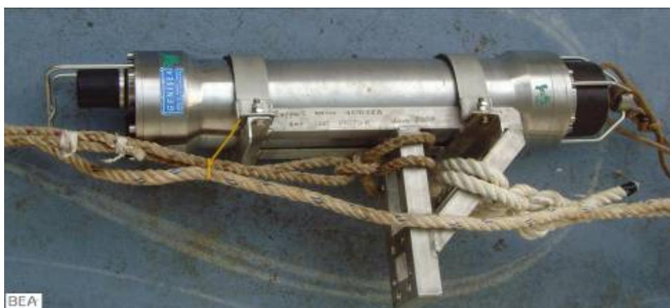
37/12 kHz acoustic repeater
