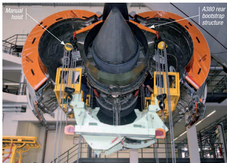
Figure 3 A380 bootstrap structure
