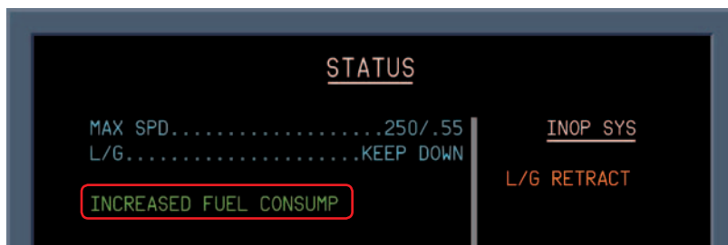
Figure 3 STATUS page of L/G GEAR UPLOCK FAULT
