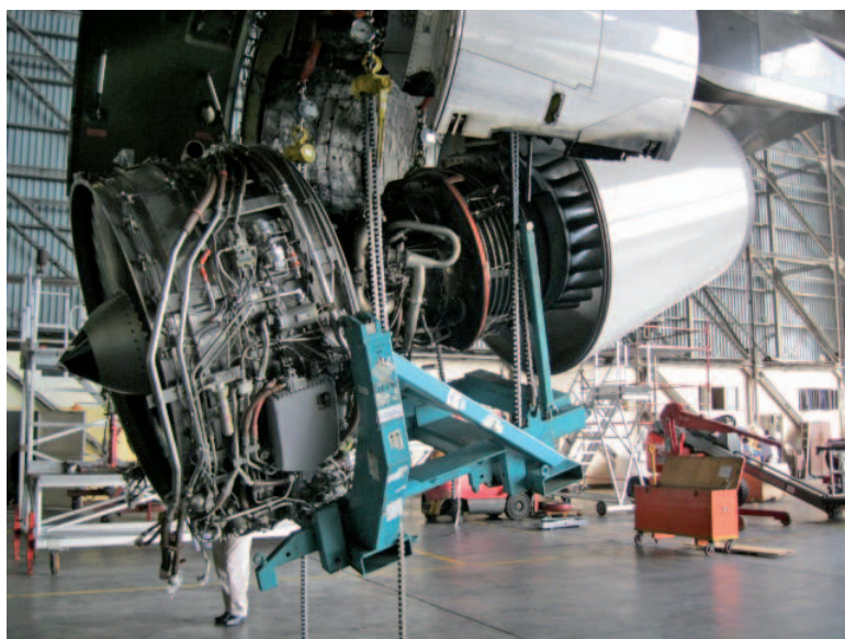
Figure 2 consequence of disengaged chain pulley
