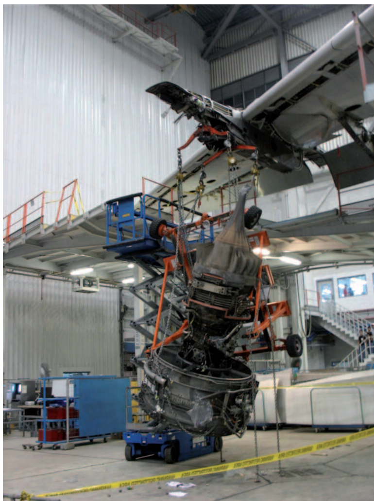
Figure 1 Consequence of failed bootstrap
