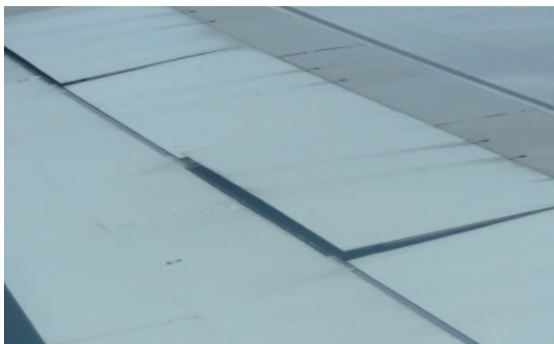
Figure 1C Illustration of spoiler drift on an A330
