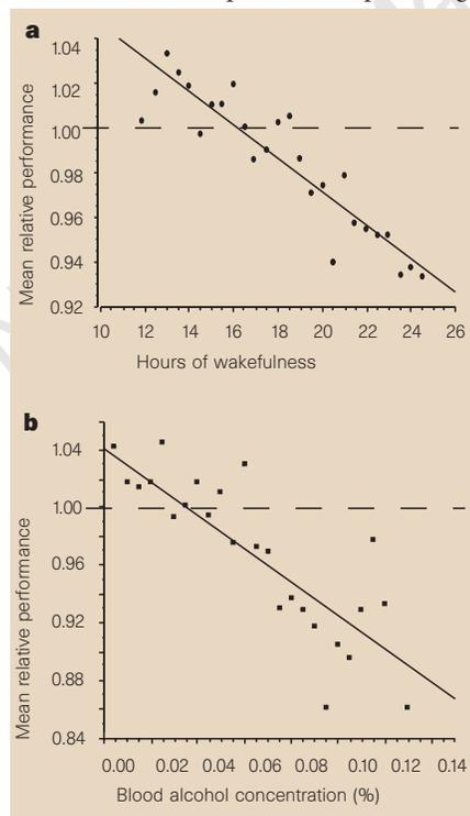
**Figure 1** Scatter plot and linear regression of mean relative performance levels against: **a**, time, between the tenth and twenty-sixth hour of sustained wakefulness ( $F_{1,24}=132.9$ ,  $P<0.05$ ,  $R^2=0.92$ ); and **b**, blood alcohol concentrations up to 0.13%, ( $F_{1,24}=54.4$ ,  $P<0.05$ ,  $R^2=0.69$ ).
