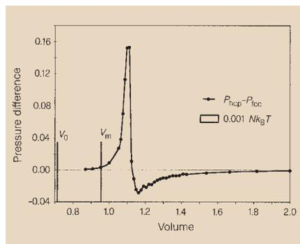
**Figure 1** Latest molecular dynamic data for the pressure difference as a function of volume at constant temperature,  $\Delta P(V)_T$ , between the h.c.p. and f.c.c. single-occupancy-cell crystal structures for hard spheres;  $V_0$  is the close-packed crystal volume and  $V_m$  is the volume at melting. The area under this curve is the Helmholtz free-energy difference between the two crystal structures at close packing in units of  $Nk_B T$ .
